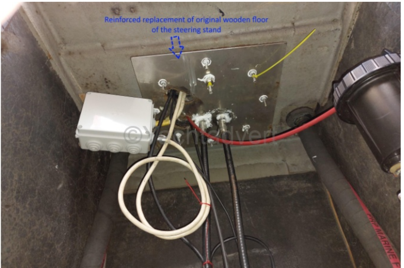
Reinforced replacement of original wooden floor of the steering stand
